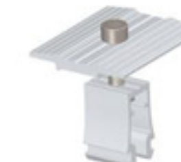
AS-AMC Adjustable mid clamp 50mm width Material: aluminum 6005-T5 Application: Framed panel thickness 30-50mm, aluminum rail - n module series
