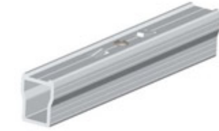
AS-RS-07 7# Rail splice L150*W20.3*H21.7mm Material: aluminum 6005-T5 Rivet 1pcs
