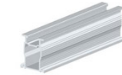
AS-R-07B Rail 7B# W32.30*H38.00mm Material: aluminum 6005-T5
